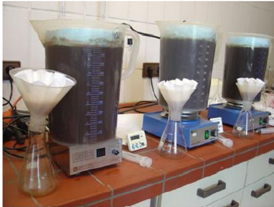
Figure 3. Set-up for ex-situ activity tests in the lab (left) and measured removal of N-compounds (right)
