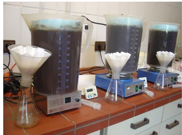
Figure 3. Set-up for ex-situ anammox activity tests in the lab (3b; right) and measured removal of N-compounds (3a; left)
