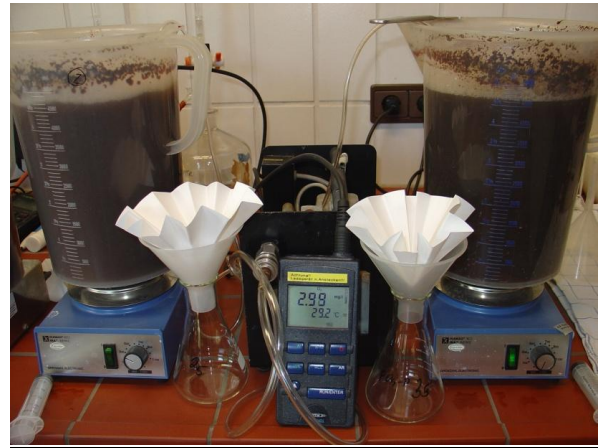
Figure 4. Set-up for ex-situ AOB-activity tests in the lab (4b; right) and measured OUR (4a; left)
